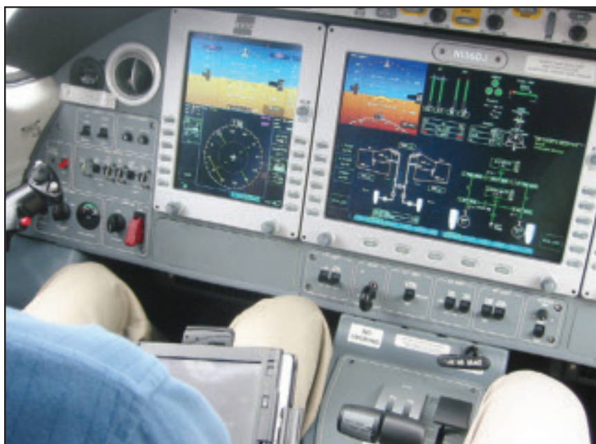
A closer look at the digital flat panel displays of the Eclipse 500 cockpit. (Oscar Garcia)
